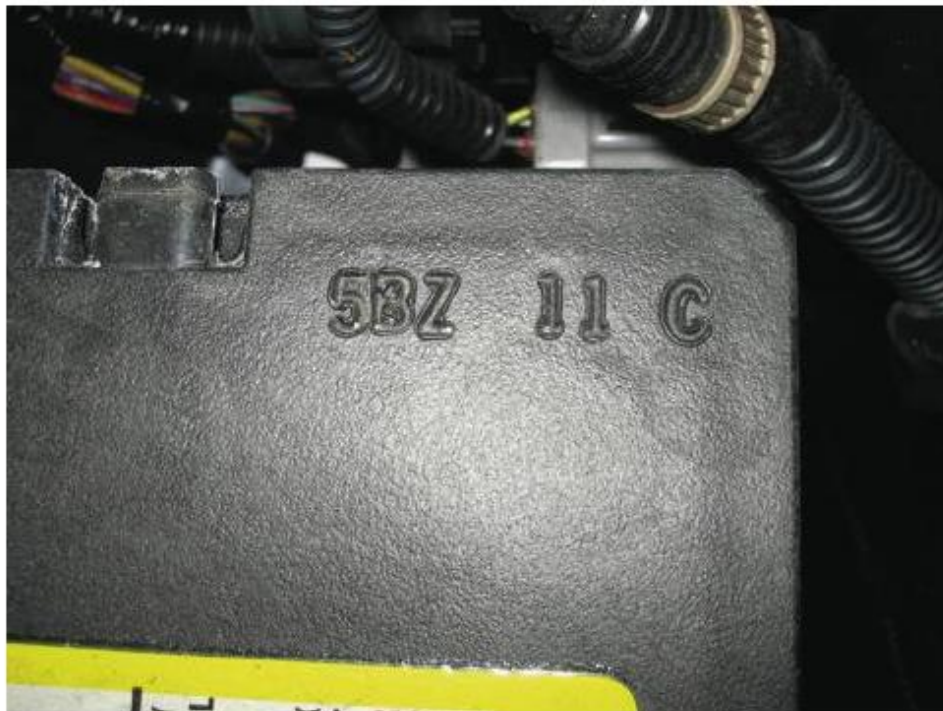
FIGURE 51-15 The code on the Delphi battery indicates that it was built in 2005 (5), in February (B), on the eleventh day (11), during third shift (C), and in the Canadian plant (Z).
